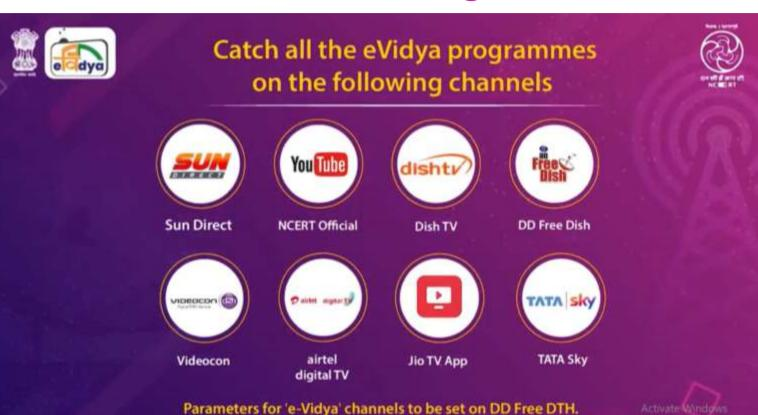
Satellite: GSAT 15(93.5 degree East) 2. Receive freq.: 11670MHz 3. Symbol Rate: 29500KSPS 4. Polarity: Vertical
